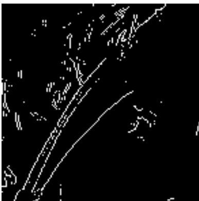
Figure 8: Edge detection using the first derivative and cubic spline model; exact implementation based on NONCIIR method.
