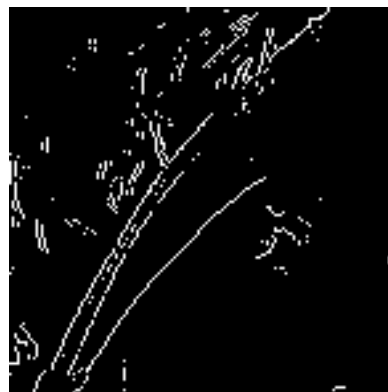
Figure 9: Edge detection using the first derivative and cubic spline model; approximation based on 5KFIR method, \beta = 1.76 .
